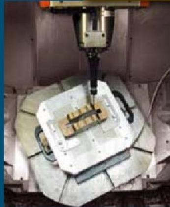
USINAGE UGV 5 AXES
