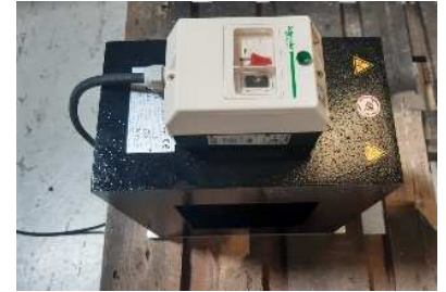
Special degaussing tunnel. Special demagnetizer with electric box on upper face.
