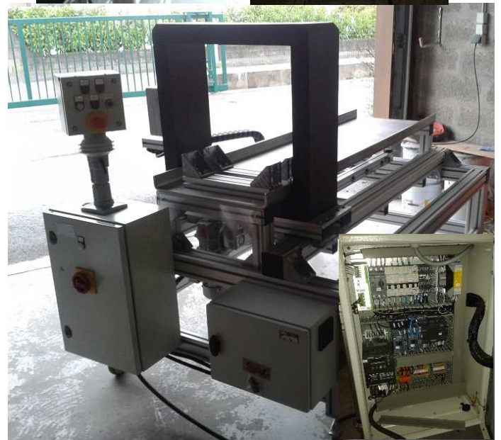
Electric box examples. Possibility to have the push button directly on the electric box or on a remote box. All our electrical boxes are made according to the standards in force and in the rules of art.
