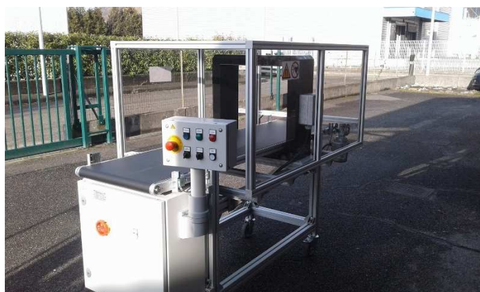
Example of a machine with automatic placement of the parts in the degaussing tunnel for the degaussing cycle and return of the parts to the initial position.
