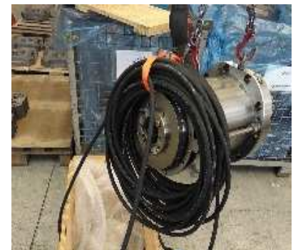
Demagnetization with cables. Very well suited for demagnetizing parts on site or for large parts.
