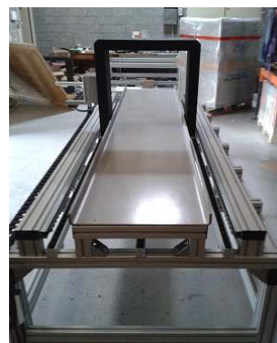
Manual demagnetizer. The tunnel demagnetizer is moving manually on handling rollers to go to the pieces placed on table.
