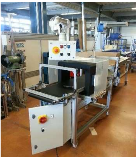
Automatic demagnetization machine. Complete automatic machine for demagnetization with remote control on articulated arm. This machine was made for a manufacturer's tool shop in aeronautics.
