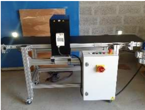
Tunnel demagnetizer with conveyor belt.
